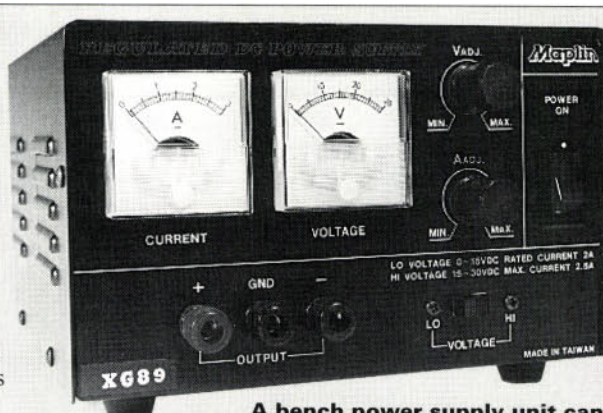
A bench power supply unit can be distinguished from an ordinary p.s.u. by its ability to vary the output voltage.
