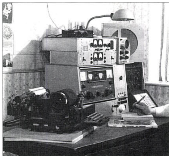
Mechanical teleprinters such as the Creed 7B in use (then) in G8CDW's station have faded away, and new techniques required a name change for the original British Amateur Radio Teleprinter Group. They are now known as the British 'Teledata' group (see text).
