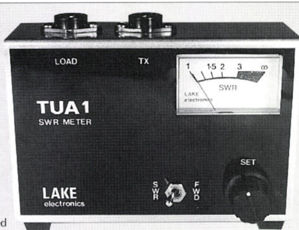
The Lake TUA1 is a single meter s.w.r. bridge, which is available in kit form from Lake Electronics.
